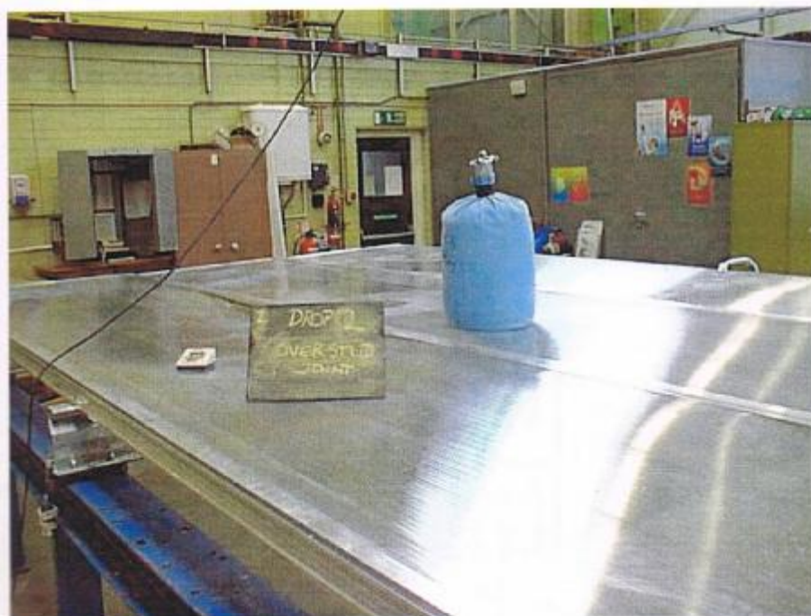
Figure 6. At a point over a joint in the threaded bar within the panels.
