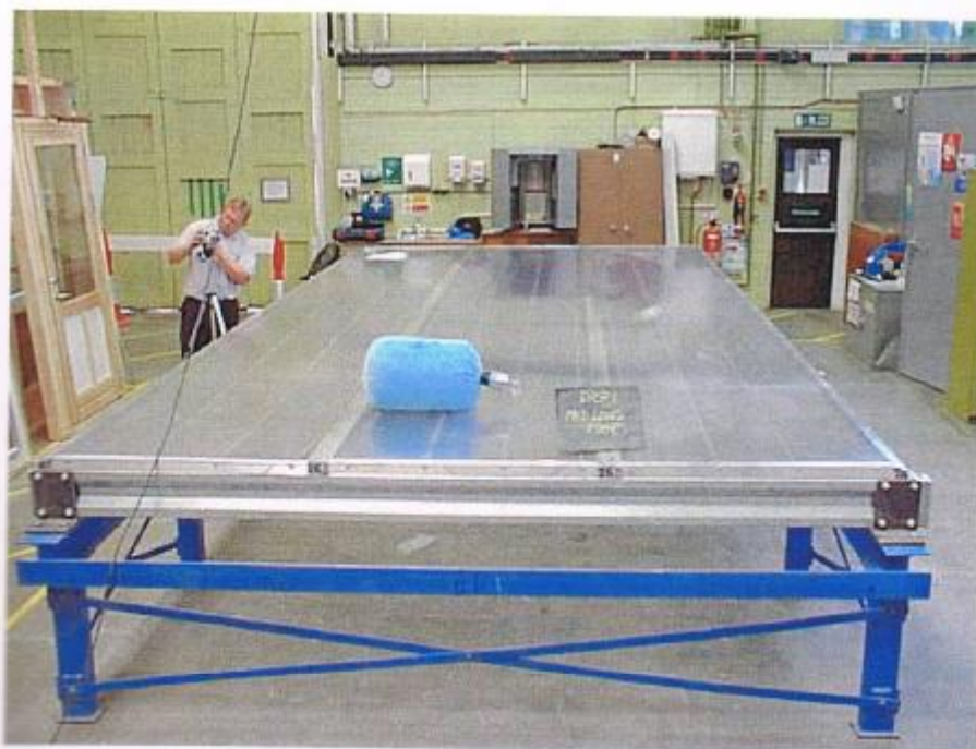
Figure 2. After the first drop at a point centre span between purlins close to a long edge of the panel
