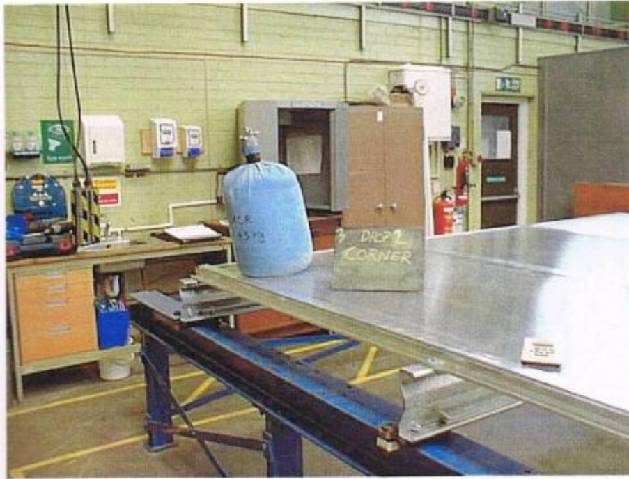
Figure 4. Third repeat test to a corner of a roof light panel
