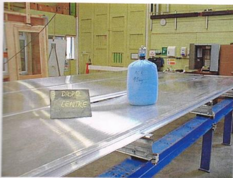
Figure 3. After the third repeat test to the centre of a roof light panel between purlins
