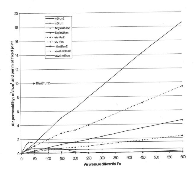
Figure A1. Air permeability per m² and per m of fixed joint under positive and negative air pressures and showing the averages of positive and negative air permeability measurements
